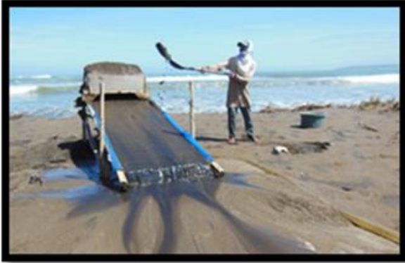
Step1 - Dousing sand with water using a parudan
