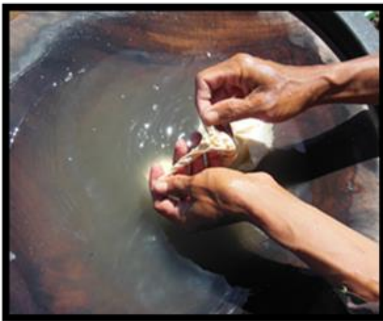
Step 3 - Squeezing the gold-mercury amalgamation - ngadulang
