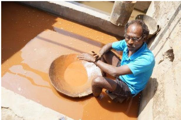
**Panning the crushed ore**
