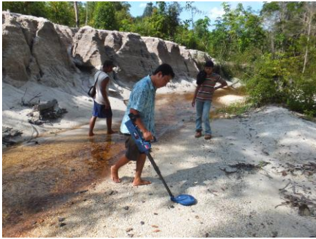
Local miners testing a Minelab detector that is also waterproof for use along river and streambeds (Model SDC 2300)
